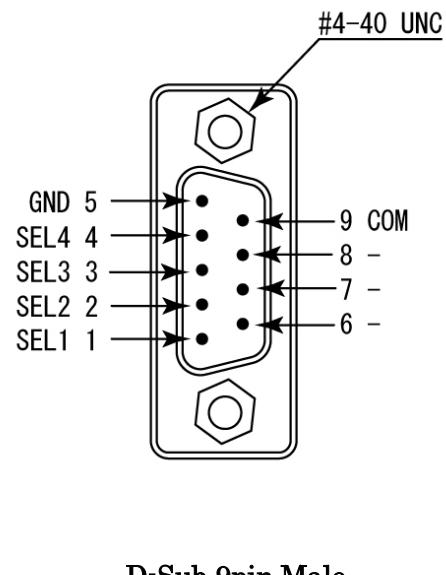
\* #4-40 UNC screws are mounted by factory setting. You can change them to attached M2.6 screws.
