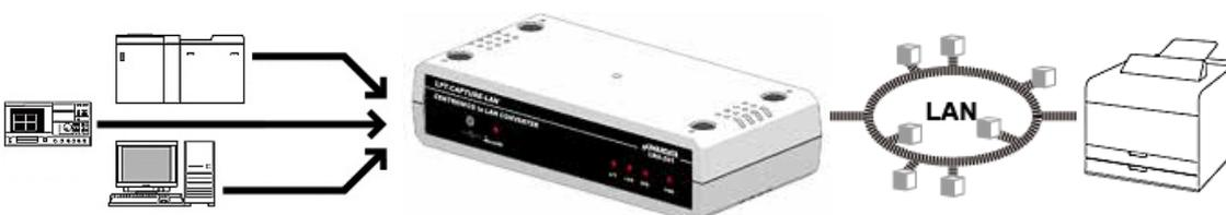
Print Centronics input data directly by relaying the data to LAN printer. To print properly, the input data should be suitable for the printer.
