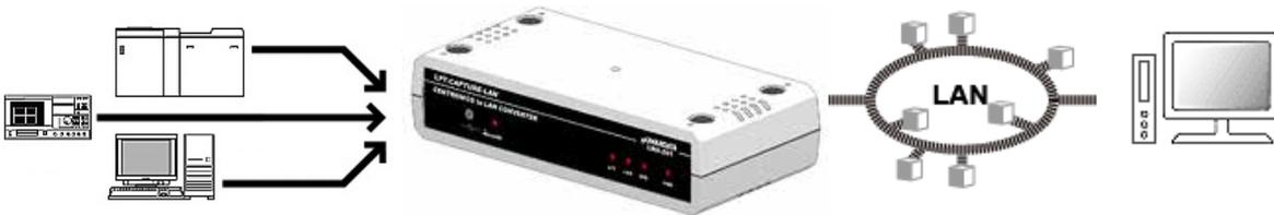
Capture parallel signal from devices which have general printer interface via a local area network.
