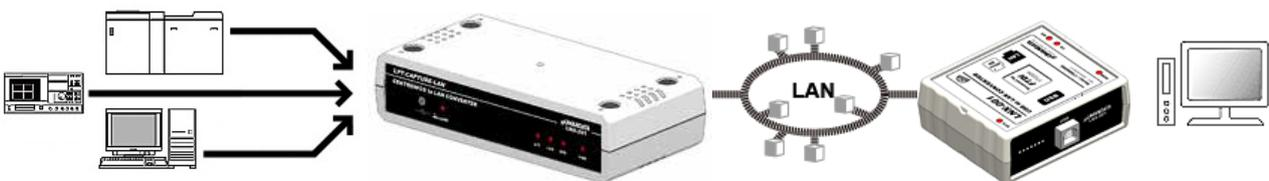
Capture parallel signal by USB interface from devices which have general printer interface via a local area network. For communication, FTDI virtual COM port and D2XX-API can be used. No need knowledge of network for the programming. LNX-001 is a USB to LAN converter.
